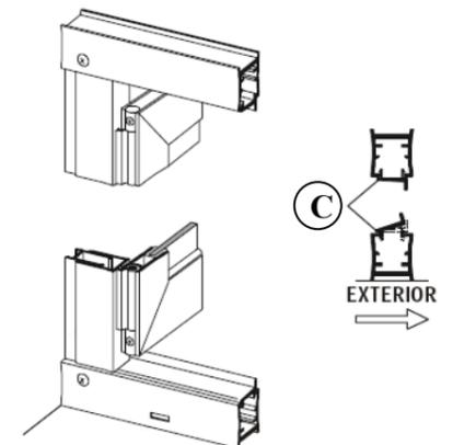
**4** Pull the bottom of the hinge jamb [A] tight to the curb filler [C] and plumb the jamb. Drill two 1/8" holes through the hinge jamb and into the wall jamb as shown in the illustration. Drill a third hole centered between the two. Enlarge the outer holes for screw clearance with a 3/16" bit. Attach the jambs with three #8 x 1/4" truss head screws [D].
