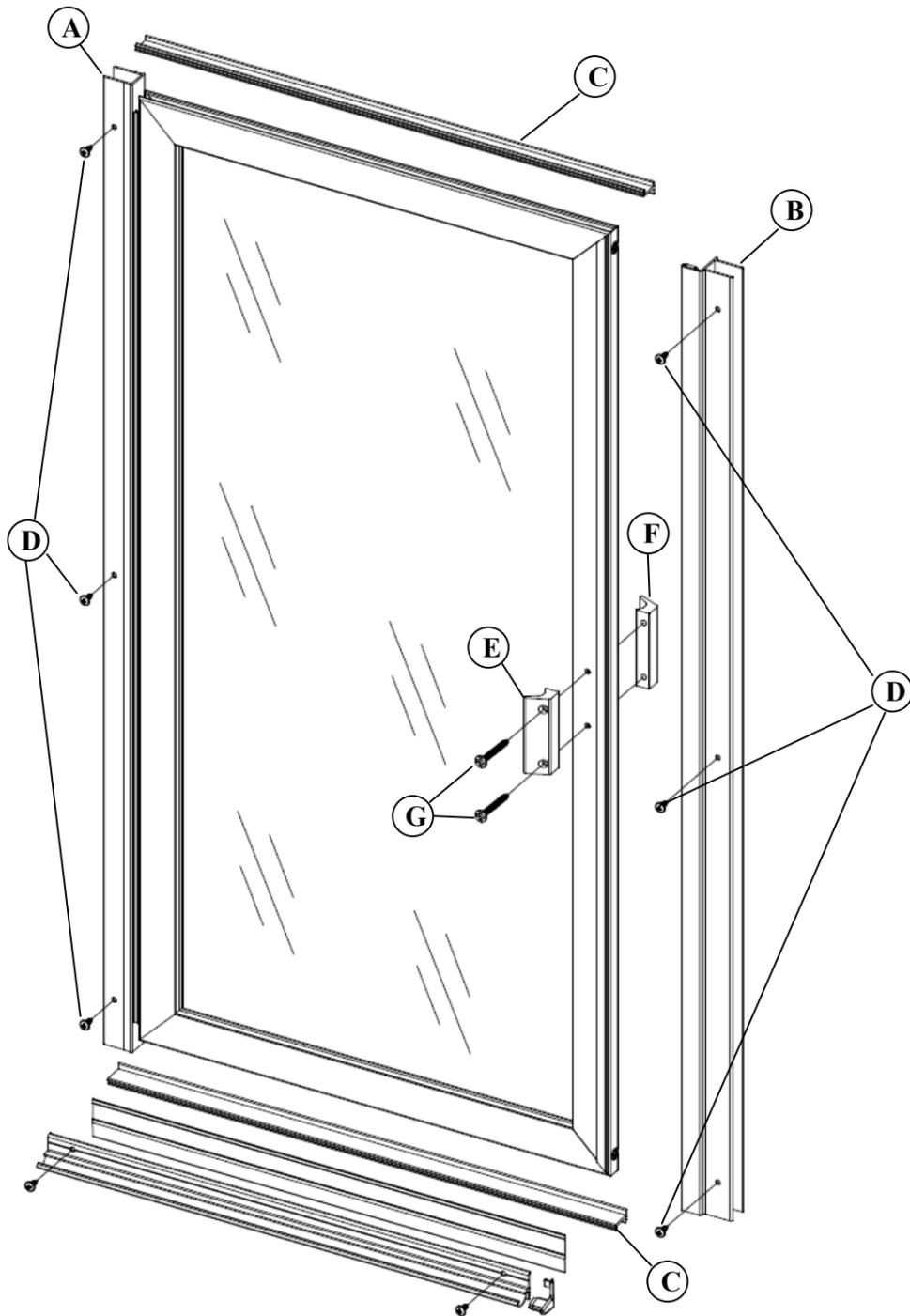
Installation Tools Required: Tape Measure, Masking Tape, Level, #2 Phillips Screwdriver, Drill with 1/8" and 3/16" bits, mallet or hammer, wood block, razor or sharp knife, hacksaw, pencil, clear silicone caulking.
