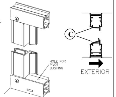
**4** Pull the bottom of the pivot jamb [A] tight to the curb filler [C] and plumb the jamb. Drill two 1/8" holes through the pivot jamb and into the wall jamb as shown in the illustration. Drill a third hole centered between the two. Enlarge the outer holes for screw clearance with a 3/16" bit. Attach the jambs with three #8 x 1/4" truss head screws [D].
