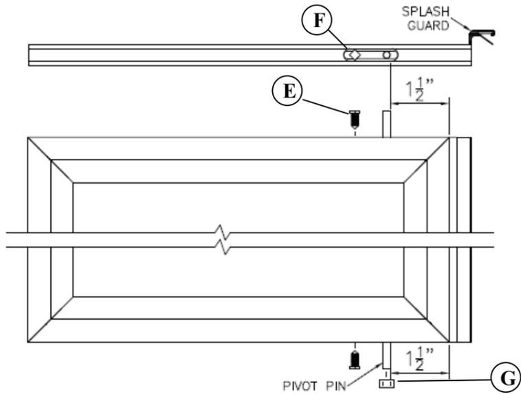
For drip rail installation refer to separate instruction sheets Adjustable Drip Installation or Standard Drip Installation.
