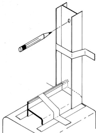
**4** Replace one wall jamba and attach to the wall by pressing a nylon spacer [E] over two #8 x 1-1/2" truss head screws [D] and insert through the top and bottom holes. Install a third screw in the center hole. Check for plumb before tightening the screws. Repeat for the other wall jamba.
