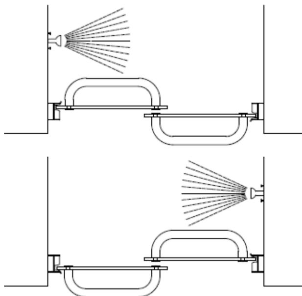
**10** Locate the bottom guide **[P]** in the center of the track with the interior panel positioned as shown. Drill two mounting holes in the track with a 7/64" bit using the holes in the guide and the V-groove in the track to locate properly. Attach with two #6 x 3/8" pan head screws **[Q]**.
