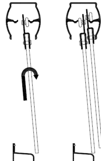
**6** Attach a roller bearing **[G]** to a hanger bracket **[I]** with a #8-32 x 3/8" hex washer head screw **[H]** as shown. Make sure the bearing is located on the side of the fin with a recess as shown in the illustration.
