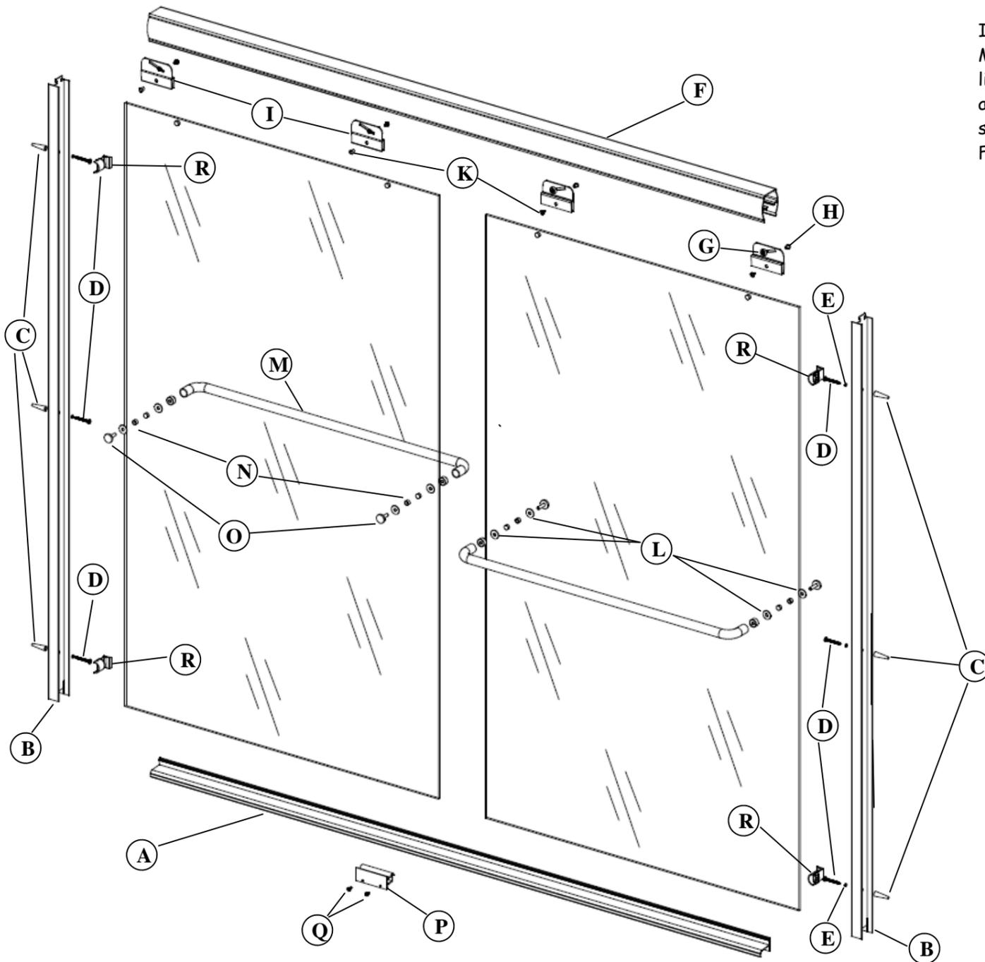
**1** Measure the wall-to-wall opening at the center of the tub rim or shower curb. Cut the track [A] 1/16" short of this dimension. Center the track as shown and use masking tape to mark the edges and secure to the tub or shower
