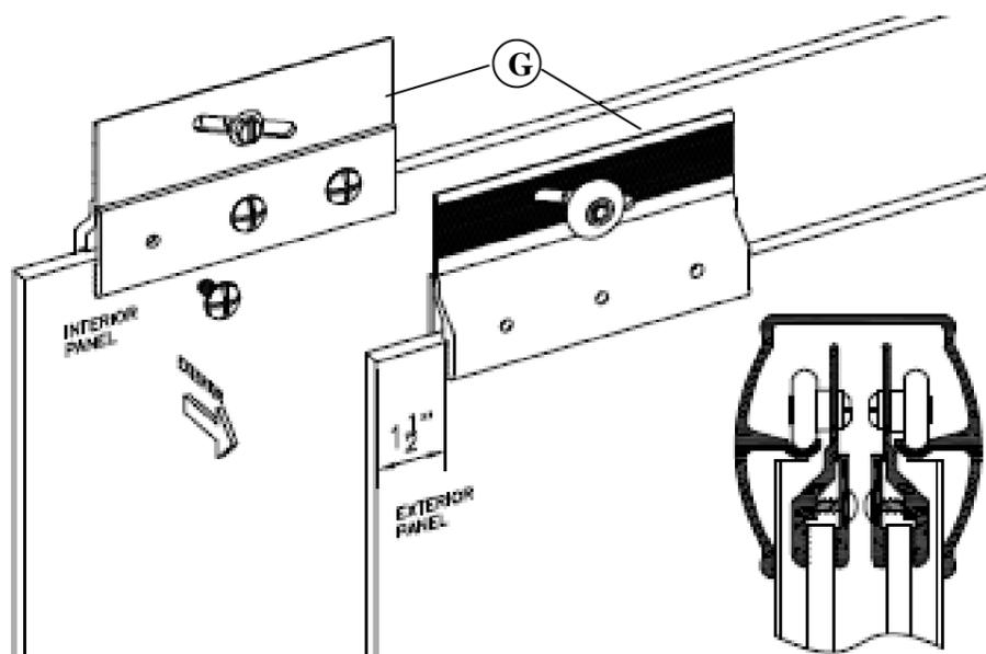
**7** Proper panel orientation should be determined before installing the door panels. To prevent leakage the interior panel should always be positioned closest to the shower head. As shown in the illustration below.
