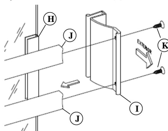
**10** At the center of the interior panel press two vinyl shims [H] over the glass then press two finger pulls [L] over the shims as shown in the illustration. Note that the longer pull handle must be to the interior of the unit as shown in the illustration in step #7.
