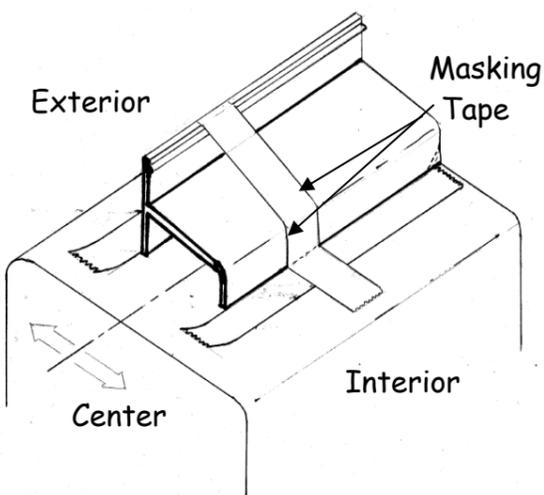
**3** Remove the parts and drill 1/8" holes approximately 1 inch deep in each wall in the marked locations. In tile or marble walls, it may be necessary to drill 3/16" holes and insert the plastic wall plugs [C]. Using a caulking gun and a good grade of silicone, run two continuous beads of sealant inside the masking tape and inside the corners. To ensure a tight fit, force a slight downward bow in the tub track. Carefully replace the track and press firmly into the sealant.
