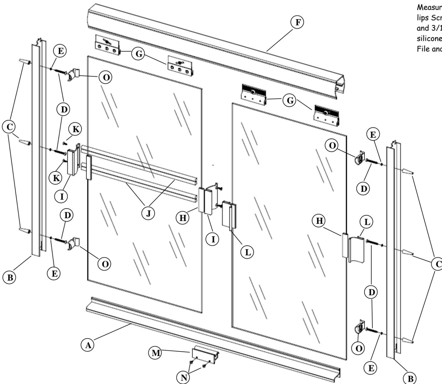
**1** Measure the wall-to-wall opening at the center of the tub rim or shower curb. Cut the track [A] 1/16" short of this dimension. Center the track as shown and use masking tape to mark the edges and secure to the tub or shower
