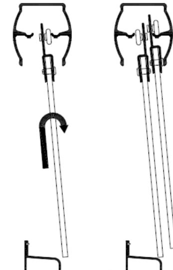
**9** At the center of the exterior panel press two vinyl shims [H] over the glass then press two towel bar brackets [I] over the shims as shown in the illustration.
