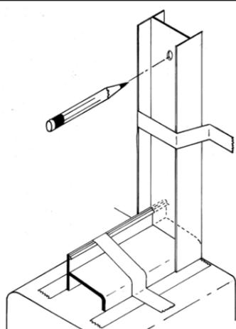
**4** Replace one wall jamb and attach to the wall with two #8 x 1-1/2" truss head screws [D] through the top and bottom holes. Press a nylon spacer [E] over a third screw and install in the center hole. Check for plumb before tightening the screws.
