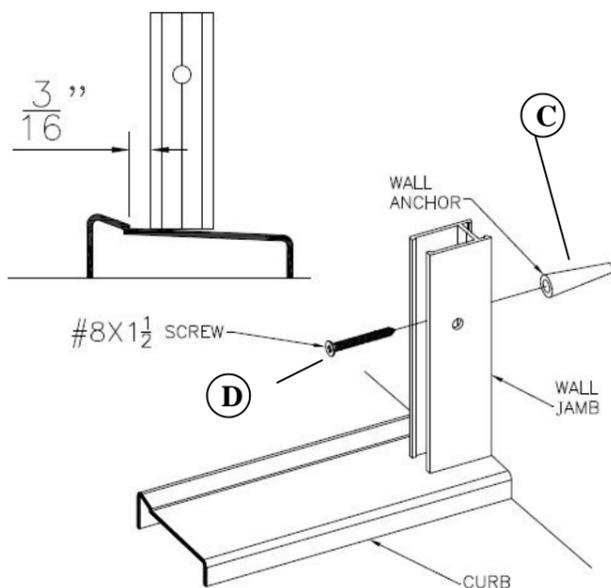
For tile or marble walls drill six 3/16" diameter holes and insert plastic wall anchors [C].
