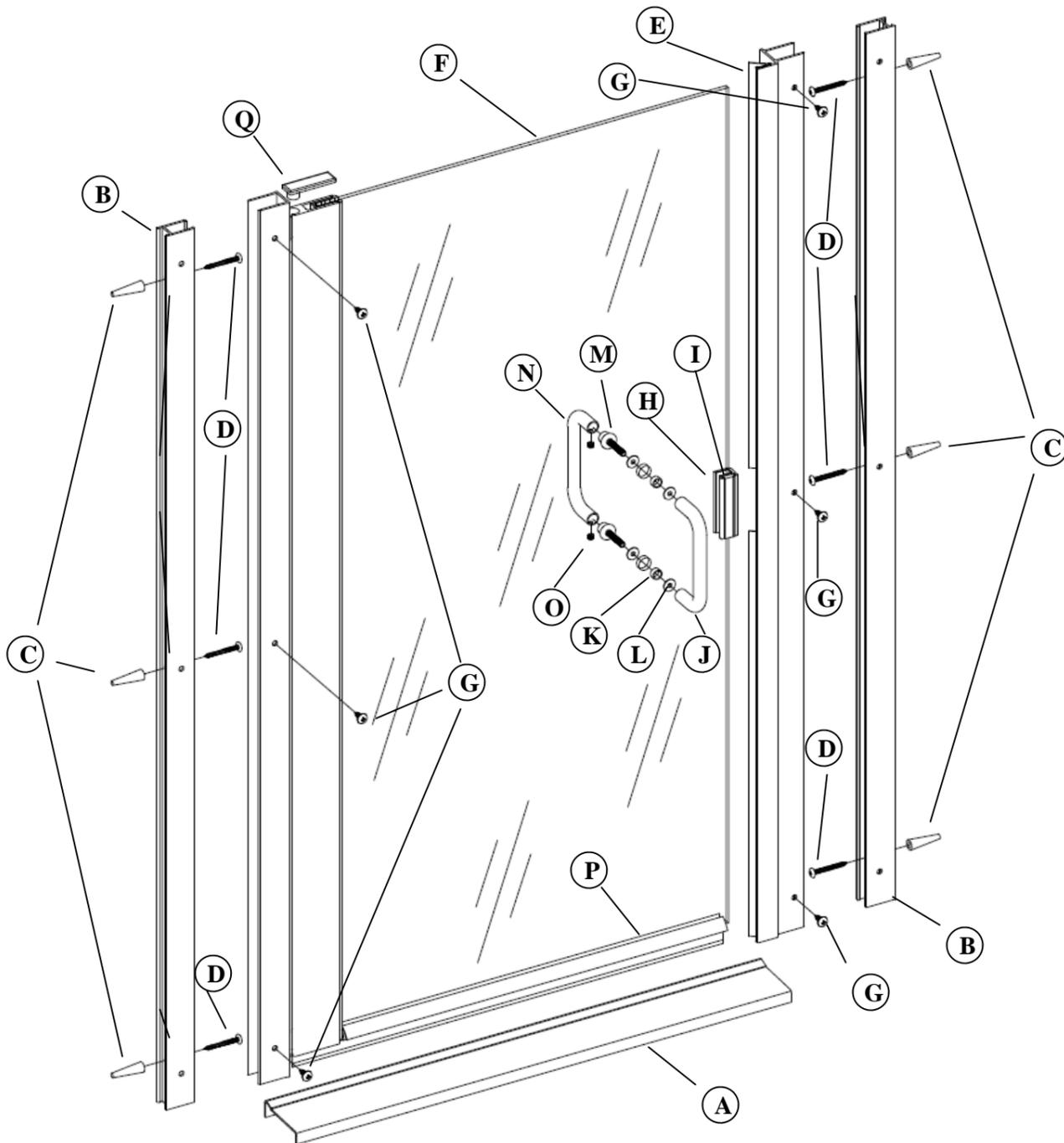
**1** The Model 30D Frameless Continuous Hinge Door is reversible and may be installed pivot-right or pivot-left. Use the diagram below to determine the correct position for your installation. For maximum waterproofing the pivot jamb should always be opposite the shower head. These instructions depict a pivot-right installation.
