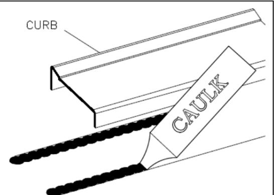
**NOTE:** Improper caulking will result in leaks.
