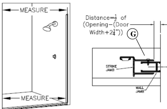
**7** Inside the enclosure, drill two 1/8" holes through the strike jamb [E] and into the wall jamb [B] 3/8" to 3/4" from the wall and approximately 1" vertically from each end of the strike jamb. Drill a third hole centered between the first two. Enlarge the three holes in the strike jamb with a 3/16" drill for clearance on the self-tapping screws. Attach the strike jamb with three #6 x 3/8" pan head screws [G].
