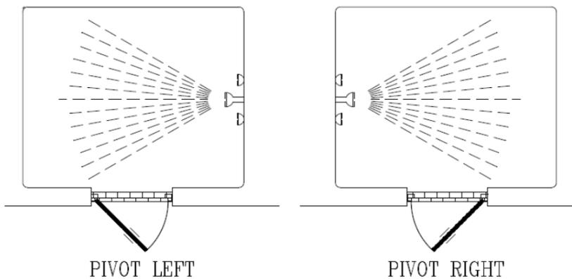
**2** **NOTE:** Obscure glass doors should be installed with the rough surface of the glass to the exterior of the unit. Make sure the glass is driven into the hinge rail a full 3/4".
