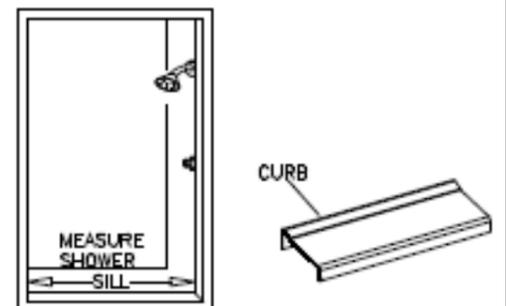
**4** Run two beads of caulk inside the pencil marks on the sill. Place the curb [A] in the exact position marked in step #2 and press it firmly into the caulking. Also caulk where the ends of the curb meet the walls. Hold curb in place with masking tape.
