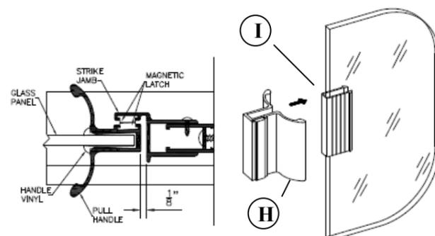
**10** Trim the flap on the clear vinyl strike jamb seal to clear the bottom door rail.
