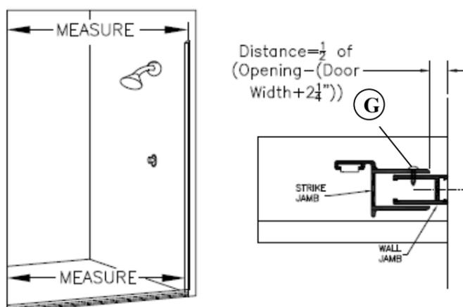
Plumb the strike jamb vertically and mark its location on the wall jamb with a pencil.
