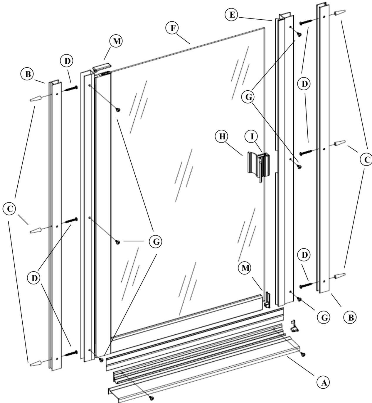
Installation Tools Required: Tape Measure, Masking Tape, Level, #2 Phillips Screwdriver, Drill with 1/8", 7/64" and 3/16" bits, hacksaw, pencil, clear silicone caulking. Optional: Miter Box, File and Center-Punch.
